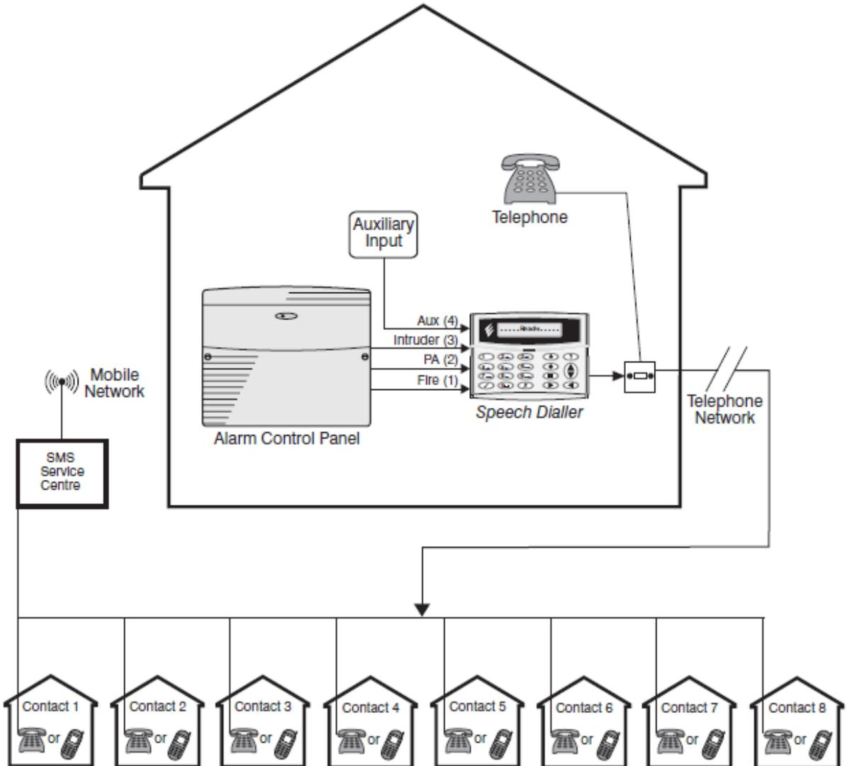
The *Speech Dialler* provides a means of communicating alarm information from an alarm control panel to a standard or mobile telephone. The unit is normally connected to an alarm control panel, which provides the necessary power and battery backup. The unit is also connected to a standard telephone line and
